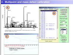
A: When the mass spectrum has been annotated (in this case using Mover7), copy the list of monoisotopic masses to the clipboard.
